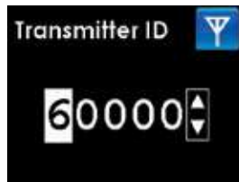
Transmitter ID setting screen, first digit highlighted
